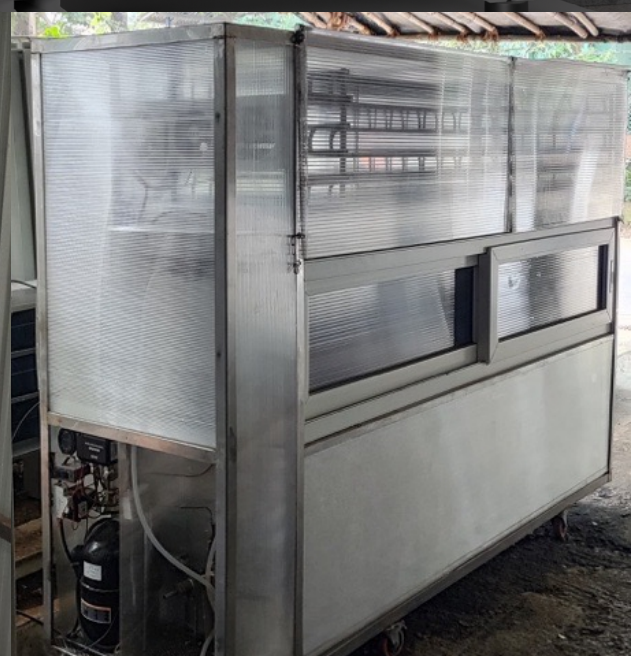
Upgraded design with larger capacity of the multi-utility heat-pump with 1m x 0,6m x 1m size.
