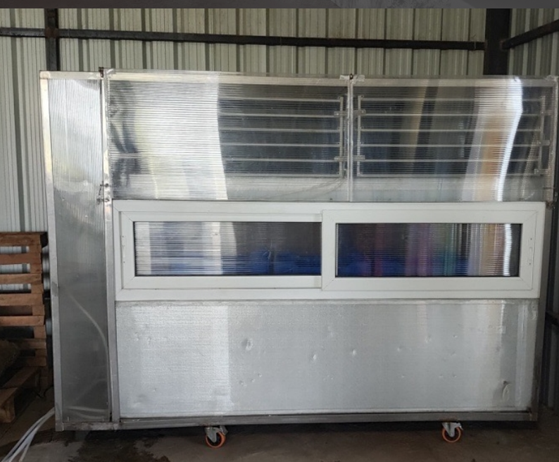
Multi-utility heat-pump for milk and water chilling and for precooling of fruits and vegetables and warm air drying for agro products
