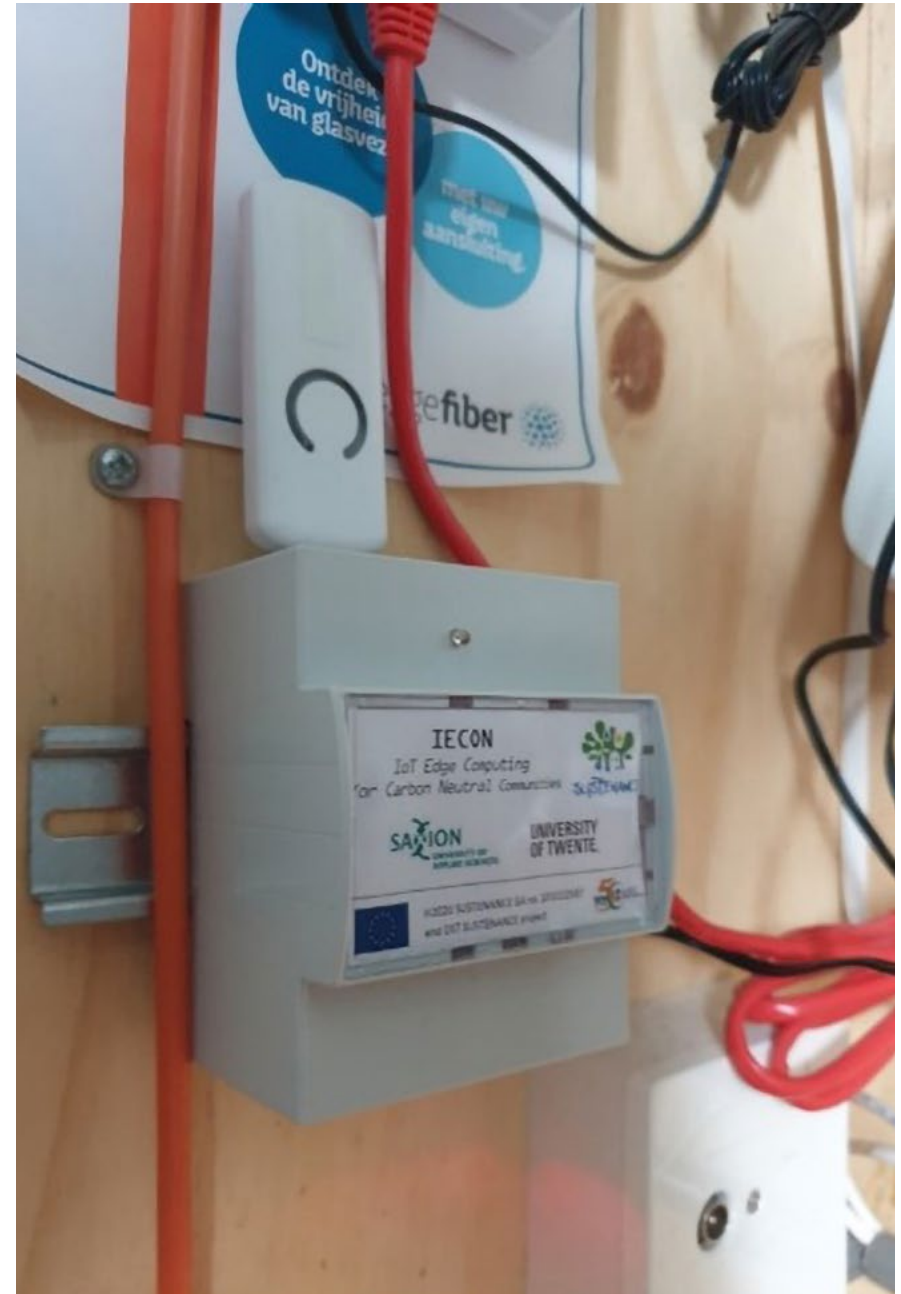
Figure 2: Installed IECON edge computer at Vriendenerf
