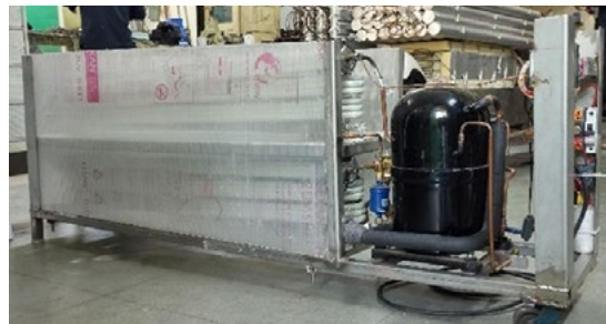
Fig. 6 Multi-Utility Heat Pump of 1.5TR rating with provision for Milk Chilling/Water Chilling, Water Heating and Drying (IIT Bombay, 2023).
