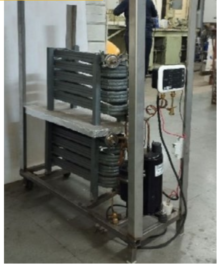
Fig. 6 Multi-Utility Heat Pump of 1.5TR rating with provision for Milk Chilling/Water Chilling, Water Heating and Drying (IIT Bombay, 2023).
