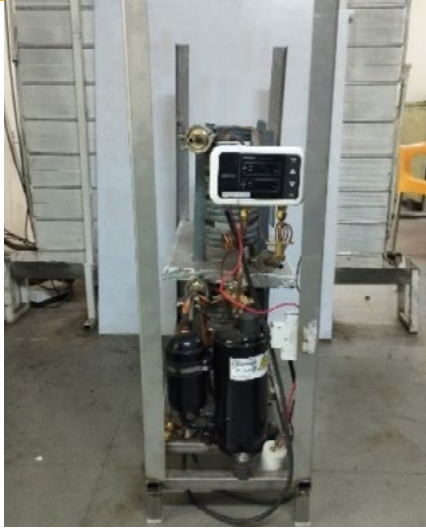
Fig. 5 Multi-Utility Heat Pump of 1TR with provision for Milk Chilling/Water Chilling, Water Heating and Drying (IIT Bombay, 2023).
