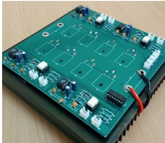
Fig. 3 Lab Prototype Development of Multi Port Converter (NIT Trichy)
