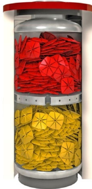
Fig. 3 PCM storage: Diameter/75 cm, height/170 cm, 500 liters storage, 440 pieces of PCM elements, capacity/15-20 kWh.
