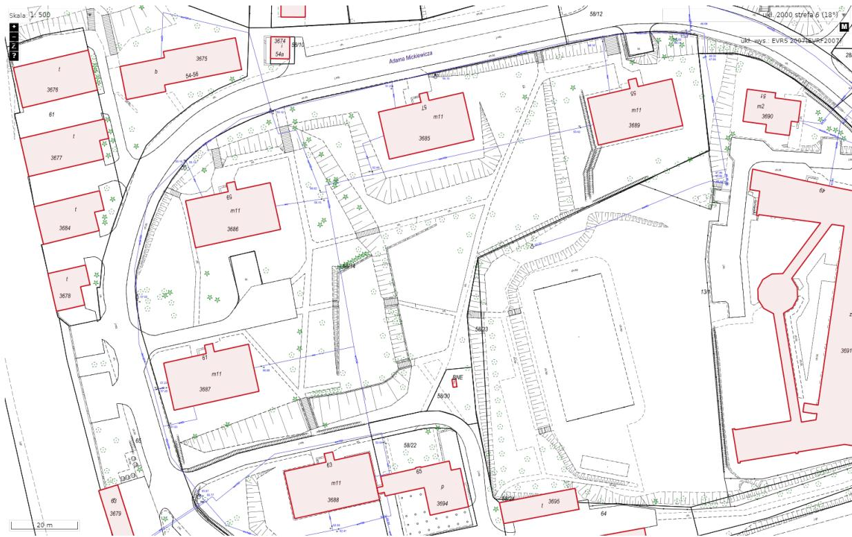
**Figure 16 Water piping over the WSM area, scale 1 : 500**
