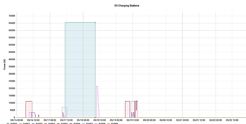
Figure 27: Charging profile of EVs connected to the SlimPark from May 16th 2022 to May 22nd 2022 (1 week).
